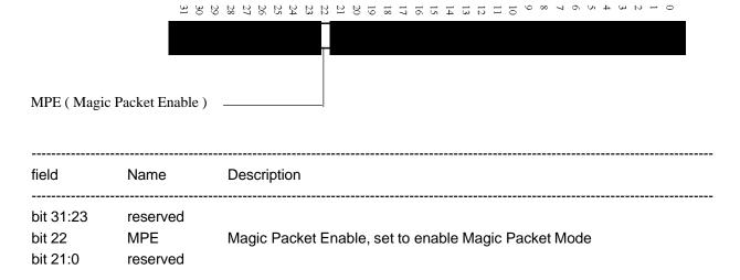
Sleep mode and MPE mode can be used seperately. When Sleep and MPE are both set, the Sleep mode dominate MPE, i.e., no magic packet can be detected since both TX and RX channel are shut off in sleep mode. In both sleep and Magic Packet mode, PWD100B will be asserted low to shut down external 100 Base-TX PHY/PMD chips. On the detection of magic packet, PWD100B pin will be asserted high.
