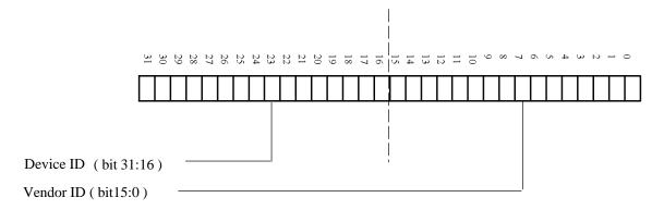
This register can be loaded from external serial EEPROM or use a MXIC preset value of "10D9" and "0531" for vendor ID and device ID respectively. Word location 3Eh and 3Dh in serial EEPROM are used to configure customer's vendor ID and device ID respectively. If location 3Eh contains "FFFF" value then MXIC's vendor ID and device ID will be set in this register, otherwise both 3Eh and 3Dh will be loaded into this register from serial EEPROM.
