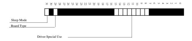
bit 31 : Sleep Mode, set to sleep mode which allows access to PCI configuration space, a hardware reset or reset to this bit can exit from sleep mode. Magic packet can be received under sleep mode if CSR16<22> ( Magic Packet Enable ) is set.
