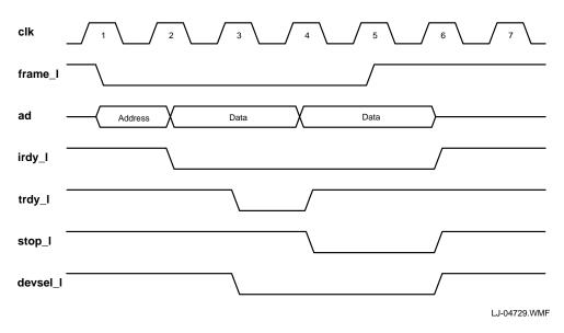
Figure 5-7. 21143-Initiated Disconnect Cycle
