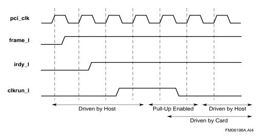
Figure 5-16. PCI/CardBus Clock—Maintaining Speed
