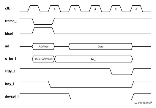
Figure 5-3. Configuration Read Cycle
