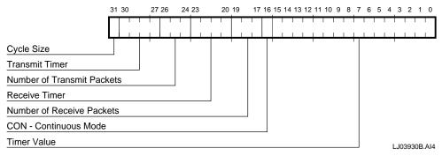
Figure 3-40. CSR11 Register Bit Fields
