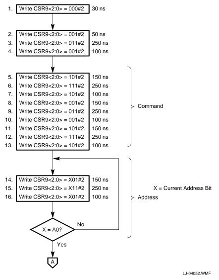
Figure 8-8. Write Cycle (Figure 1 of 2)
