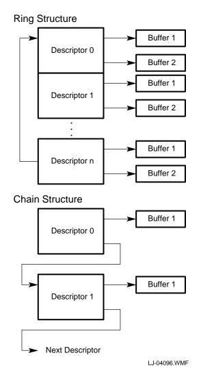
Figure 4-1. Descriptor Ring and Chain Structure Examples
