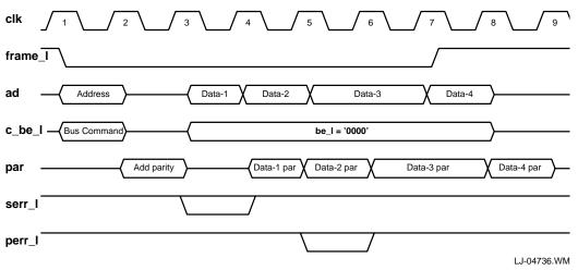
Figure 5-14. Parity Operation
