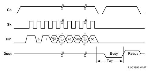
Figure 8-10. Write Operation
