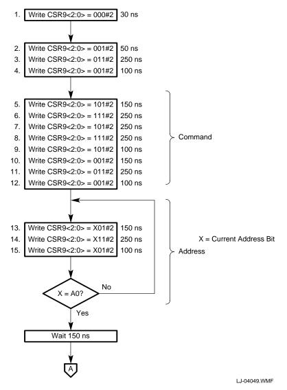
Figure 8-5. Read Cycle (Figure 1 of 2)
