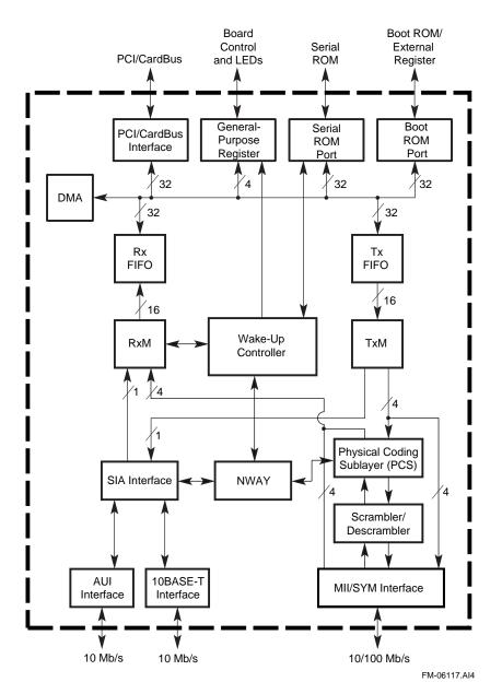
Figure 1-1. 21143 Block Diagram
