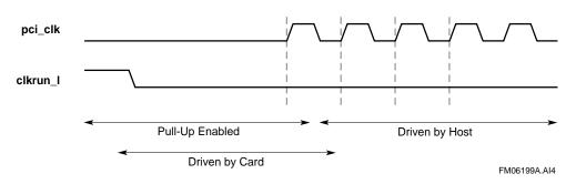
Figure 5-15 shows the PCI/CardBus clock restart or speed-up timing characteristics.
