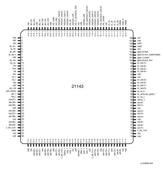
Figure 2-1. 21143 Pinout Diagram (Top View)
