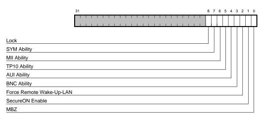
Figure 3-21 shows the CWUC register.
