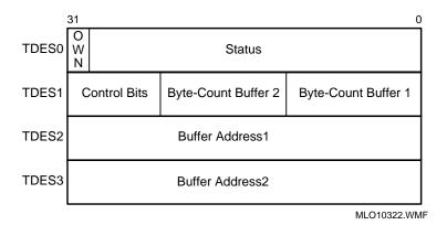
Figure 4-7. Transmit Descriptor Format
