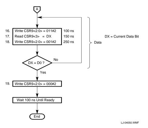
Figure 8-6. Read Cycle (Figure 2 of 2)
