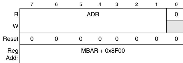
Figure 26-2. I 2 C Address Register (I2ADR)
