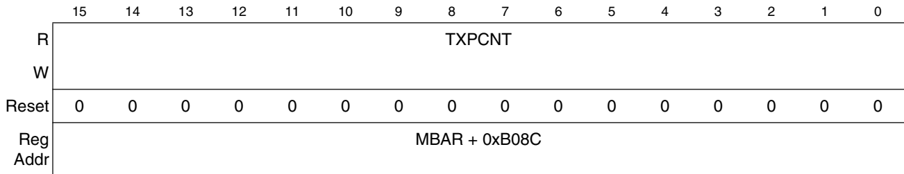
Figure 28-24. USB Transmitted Packet Counter Register (TXPCNT)
