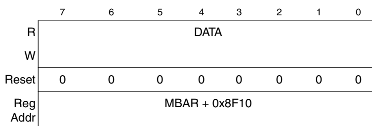
Figure 26-6. I 2 C Data I/O Register (I2DR)
