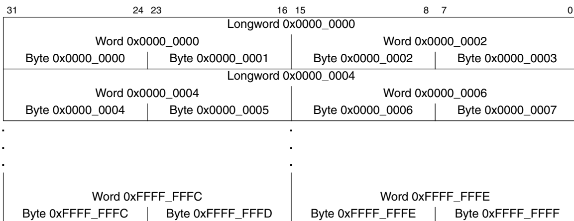
Figure 3-11. Memory Operand Addressing
